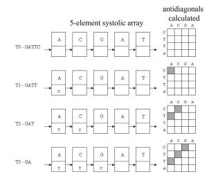
Fig. 4. Generic systolic array to calculate the dynamic programming matrix.
